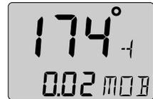
This function requires either a navigator (a NX2 GPS or NMEA navigator can be used) or a speed and compass transducer as well as a man over board (MOB) button. (See Server Manual).
