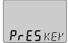
To initialise the instrument, press **SET** on all installed digital instruments, one at the time.
