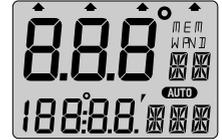
At first power on after installation, you will be asked to press **SET** (PrESkey). This will give the instrument a logical ID number on the Nexus Network.
