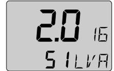
The example shows that the instrument version number is 2.0 and the given logical ID number is 16.
