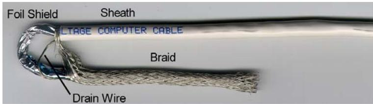
**Figure 2-6 Removing the Wire Assembly from Inside Braid**
